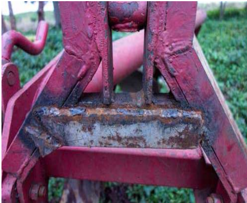
Chinese equipment welded and reinforced by pilot demonstration workers
