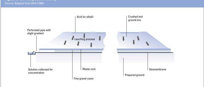
Figure 10–2. A Heap Leach Facility
