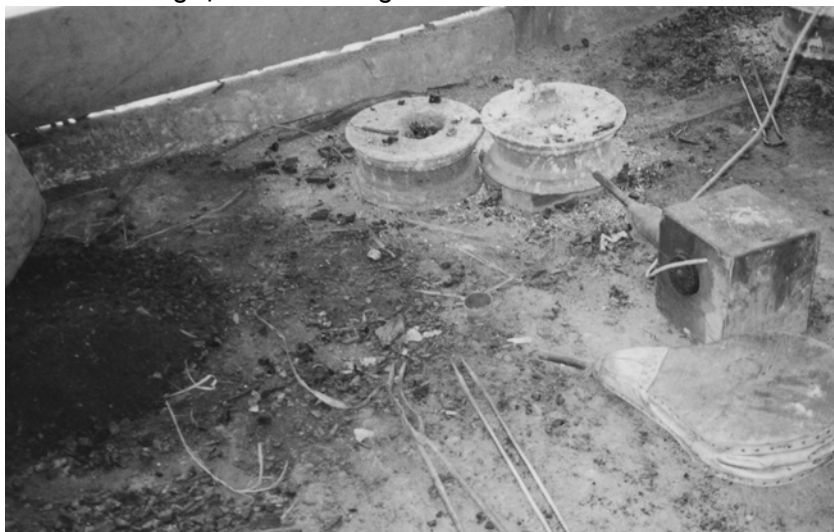
Roasting of mercury amalgam over charcoal at a small-scale Gold-mining site in Tarkwa
