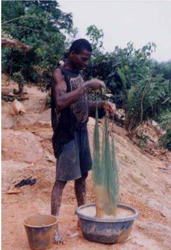
Hand washing of gold-infested sediment in a small-scale gold mining district
