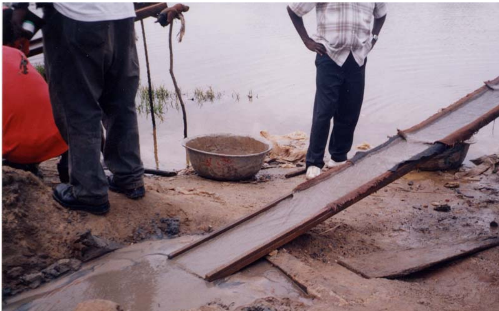
Blanket washing of sediment alongside a river in Ghana.
