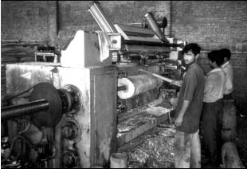
Poplar log being peeled in a local plywood factory in Uddham Singh Nagar
