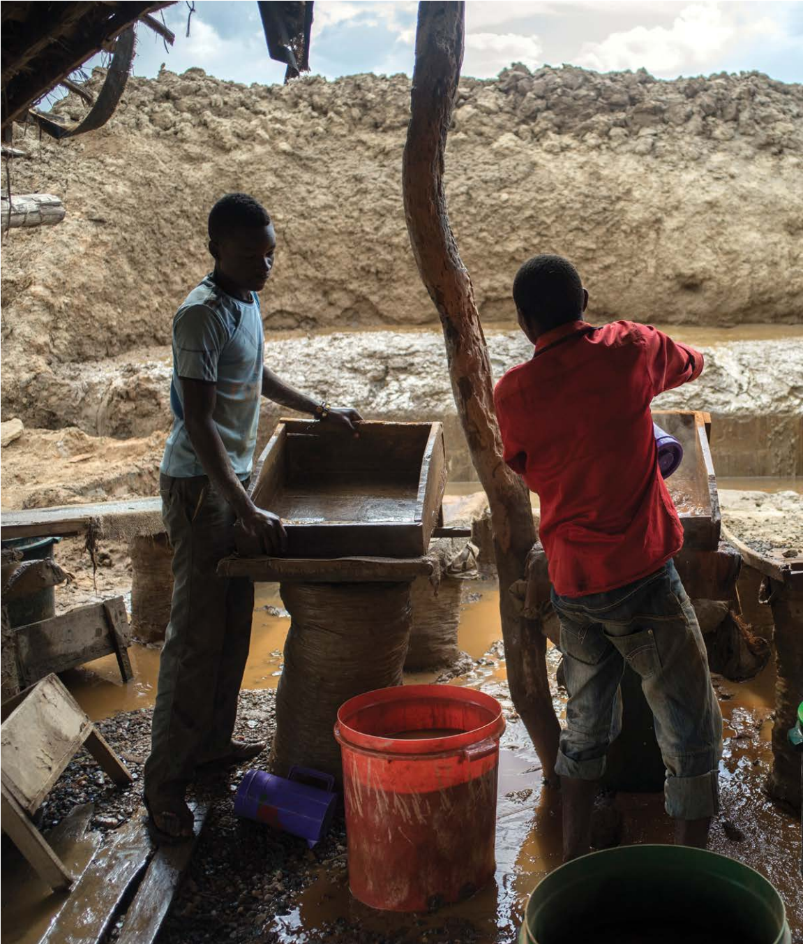
Young men pour water into a powdered mix of gold and other materials during the extraction process at Nsangano Gold Mine, Mawemeru village, Geita District, Tanzania on March 19, 2015. The gold will remain stuck to the surface of the wet towels, while the lighter materials will wash away. While effective, this method is not as profitable or environmentally friendly as more advanced techniques that omit the use of mercury. Credit: Brian Sokol/Panos Pictures
