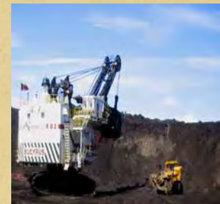
Even bigger mining shovels are used. These cost $20m each and stand seven storeys high. They can dig out 100 tonnes with one shovelful. Four shovel loads fill one truck.
