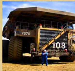
Heavy hauler mining trucks are used to move tar sand in Canada. These machines can carry up to 400 tonnes of sand and have tyres that are 15 feet high.
